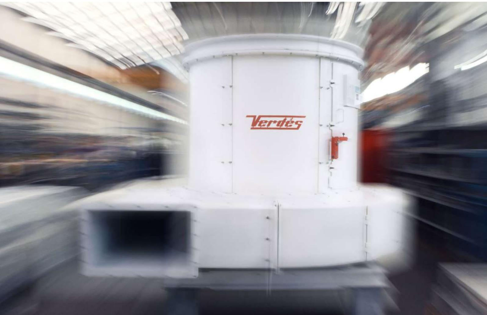
The mill has a set of pendulums with rollers at the ends that grind the material at high pressure against a grinding ring. Pressure is created from the high-speed rotation of the star from which the pendulums hang.
