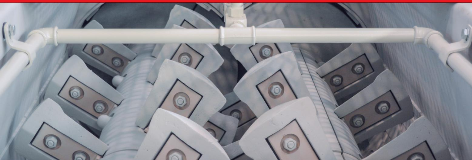
Intensive mixing of the clay body with automatic regulation of extrusion moisture levels.
