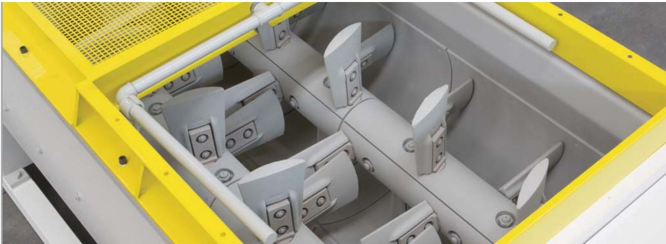
Mixing area for the homogenization of the various components, clays and additives.
