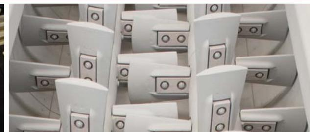
Essential equipment in the preparation process to ensure accurate and homogeneous mixing of various types of clay and powder or liquid additives. High performance based on “knife-on-knife” mixing concept.
